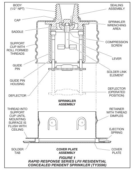
allowing the sprinkler to activate and flow water.
