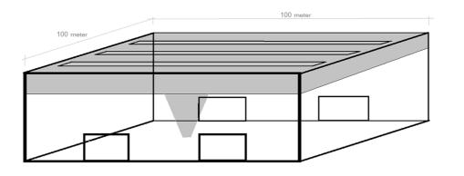
Simplified model, 2 zone simulation: 10,000 m<sup>2</sup> floor area 7 m height
