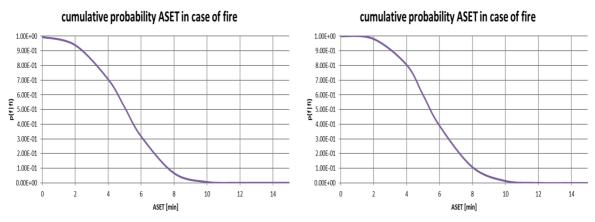
**Figure 8:** Cumulative probability distribution ASET in the corridor, criterion visibility (left: non-sprinklered reference situation; right: sprinklered situation)
