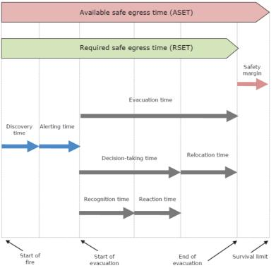
Figure 1: Safe evacuation is possible if ASET > RSET. The safety margin is the difference between ASET and RSET (Hagen et al, 2017)
