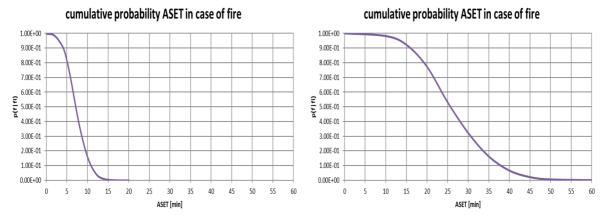
Figure 11: Cumulative probability distribution ASET in the fire compartment, criterion CO-dose (Left: non-sprinklered reference situation; Right: sprinklered situation)
