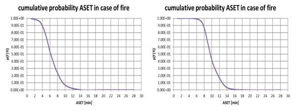
Figure 7: Cumulative probability distribution ASET in the large compartment with low ceiling, criterion visibility > 5 m (left: non-sprinklered reference situation; right: sprinklered situation)
