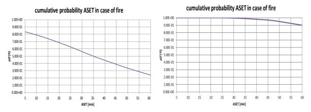
Figure 10: Cumulative probability distribution ASET in the corridor, criterion CO-dose, after opening of the fire compartment (5 minutes) (Left: non-sprinklered reference situation; Right: sprinklered situation)
