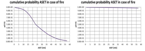
Figure 6: Cumulative probability distribution ASET in the large compartment with high ceiling, criterion smoke free height > 2,5 m (left: non-sprinklered reference situation; right: sprinklered situation)
