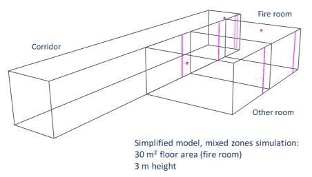
Figure 3: Corridor attached to a small compartment, mixed zones in all compartments
