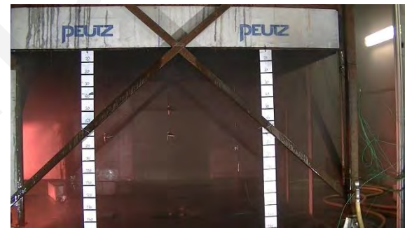
Figure 12 - Snapshot smoke layer height SH5 after 151 seconds, sprinkler active for 30 seconds
