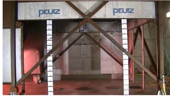
Figure 14 - Snapshot smoke layer height SH4 after 123 seconds, activation of sprinkler
