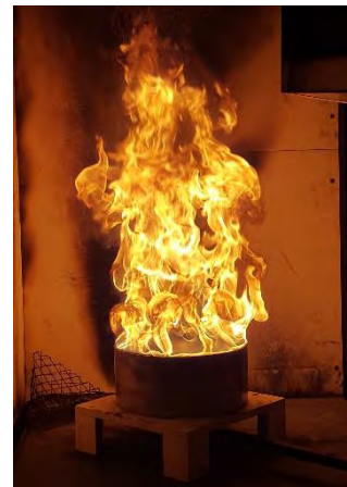
Figure 1 - Heptane/Toluene calibration procedure
