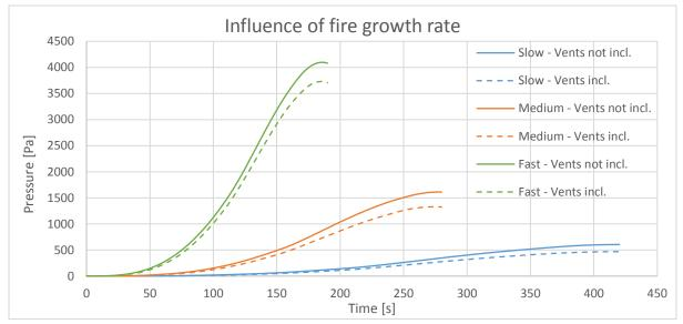
Figure 16 - Pressure increase in time for different fire growth rates, fire is located in compartment 1
