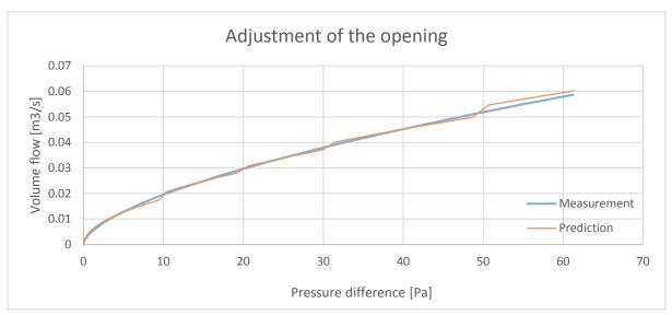
Figure 9 - Prediction of the volume flow by changing the opening for small pressure intervals
