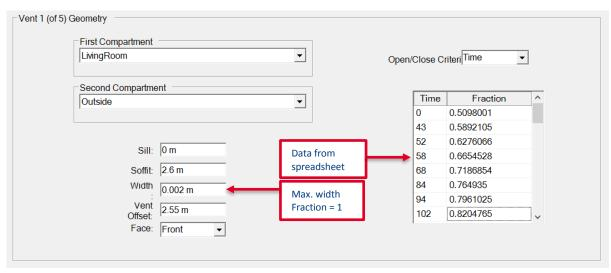
Figure 10 - Changing the opened fraction of openings in CFAST
