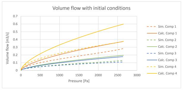
*Figure 8 - Volume flow with constant openings as calculated*
