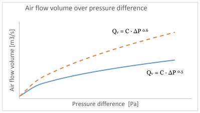
Figure 3 - Difference in air flow volume with different flow exponents
