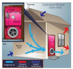
Figure 1 - Measurement setup Blower Door Test, source: (RedPoint LLC, 2017)
