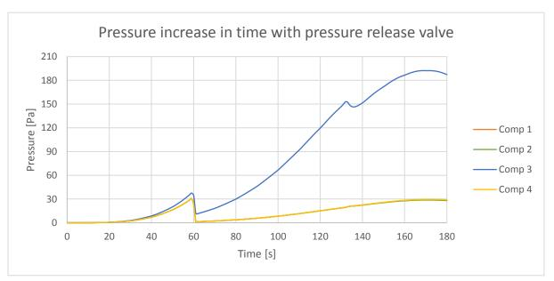
Figure 19 - Pressure increase in time, 15x25cm pressure release valve, fire located in compartment 3
