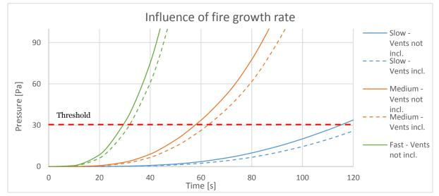
Figure 17 - Pressure increase in first two minutes for different fire growth rates, fire is located in compartment 1
