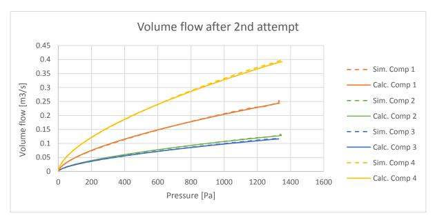
Figure 12 - Volume flow with variable openings, after 2nd attempt
