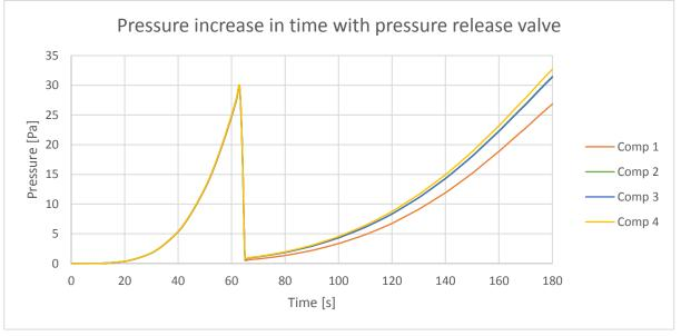
Figure 18 - Pressure increase in time, 20x25cm pressure release valve, fire located in compartment 1
