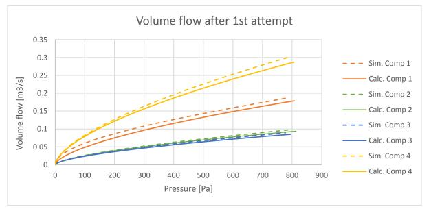
Figure 11 - Volume flow with variable openings, after 1st attempt
