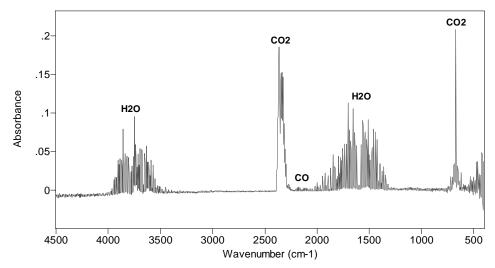
Figure 17. 1-min average of spectra for fire room during suppression in Test 4
