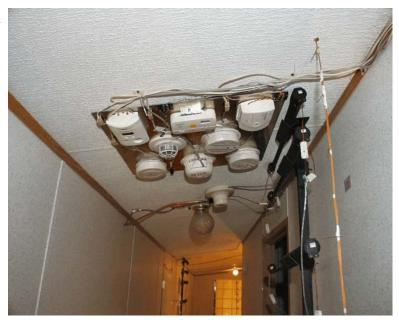
Figure 1. Sample sensor test board used during tests of residential smoke alarms
