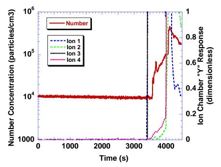
Figure 131. Smoke properties for smoldering mattress with burn room door closed SDC14
