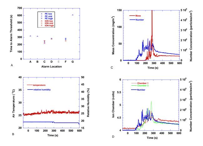
Figure 150. Toasting bread scenario - toaster on at t=0, off at 270 s. Room fan turned on
