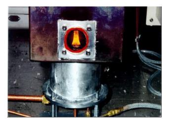
Figure 3. Propene smoke generator.
