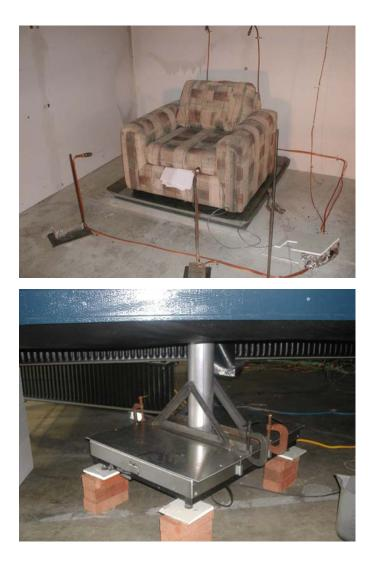
Figure 94. Example of mass loss measurement showing upholstered chair on load cell prior to one of the flaming ignition tests and load cell apparatus mounted beneath manufactured home
