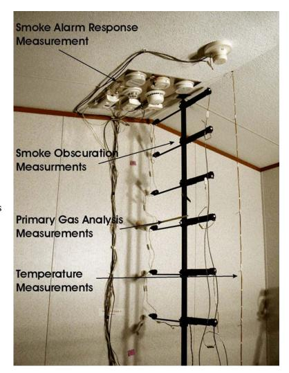
Figure 90. Sample instrumentation showing relative locations of temperature, primary gas analysis, smoke obscuration, and smoke alarm response measurements
