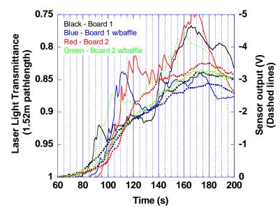
Figure 58. Ion-1 response, fan speed 12 Hz - repeat test
