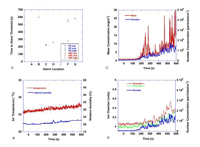
Figure 164. Frying hamburgers - three hamburgers in non-stick frying pan, floor fan on. Hamburgers in pan at t=150 s
