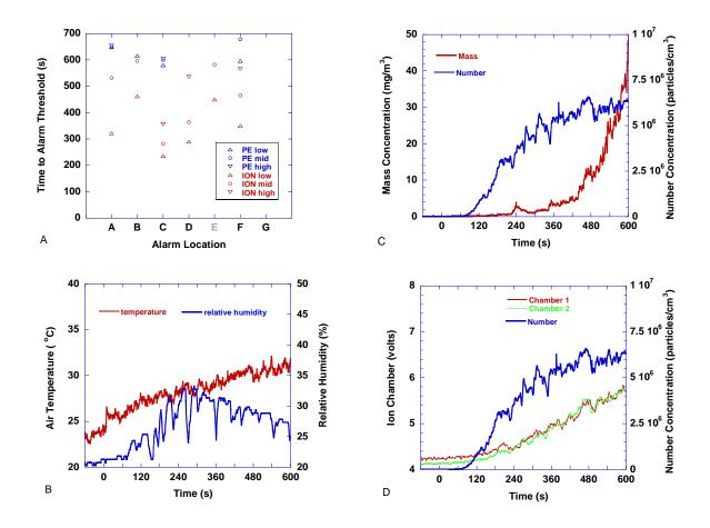
Figure 153. Frying bacon scenario - cast-iron pan, LPG hot plate, no forced flow, burner lit at t=0, bacon in pan at 60 s
