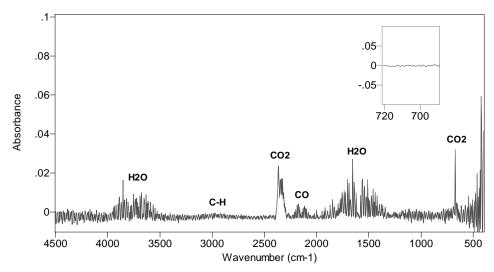
Figure 23. Average of spectra for fire room during the last 30 s of mattress smouldering (Test 14)
