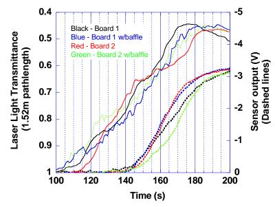
Figure 62. Ion-3 response, fan speed 5 Hz - repeat test
