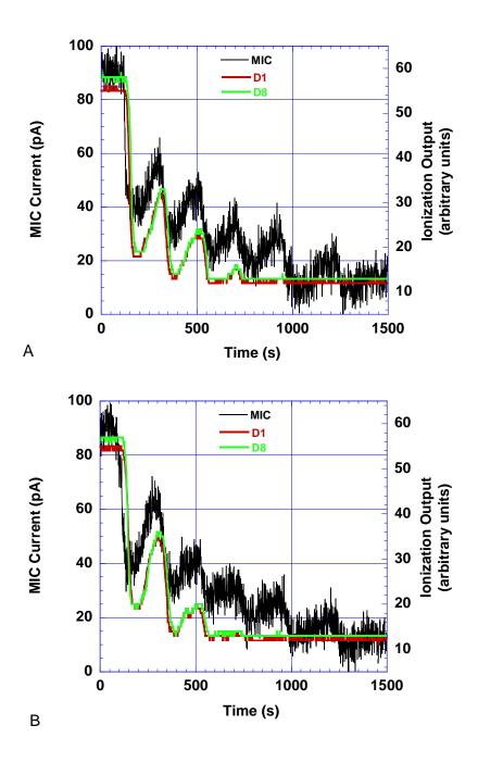
Figure 187. Ionization sensor response to cotton smolder smoke calibration test. A and B indicate repeated tests
