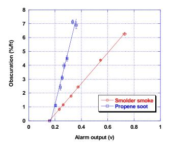
Figure 15. Calibration runs for Photo-2 alarm
