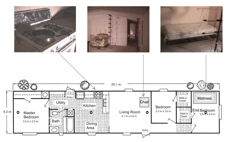
Figure 2. Plan view of a manufactured home (floor plan courtesy of NIST), fire locations (chair, mattress, kitchen stove) and FTIR gas sampling locations (☉)
