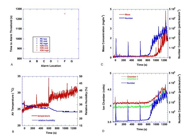
Figure 169. Bake/ broil pizza - one frozen pizza in oven set on bake and pre-heated to 350 °F, then set to broil 630 s later. Floor fan was on. Pizza in at t=0
