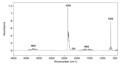
Figure 20. 3-min average of spectra for fire room during mattress flaming (Test 7)
