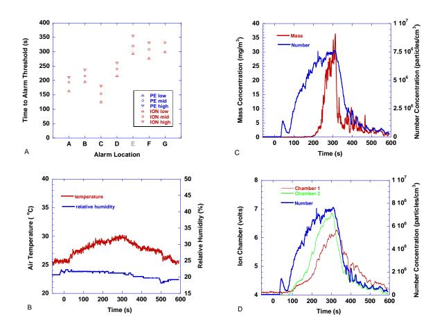
Figure 151. Toasting frozen bagel scenario – toaster on at t=0, off at 300 s. Room fan turned off
