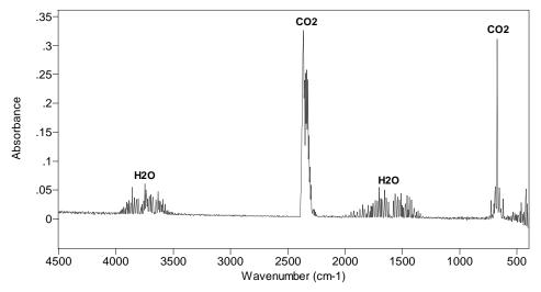
Figure 10. 1-min average of spectra at peak smoke obscuration in master bedroom(Test 2)
