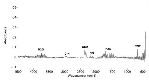
Figure 7. 4-min average of FTIR spectra (at 60 min) for master bedroom (Test 1)
