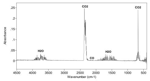
Figure 19. 2-min average of spectra for fire room during mattress flaming (Test 5)
