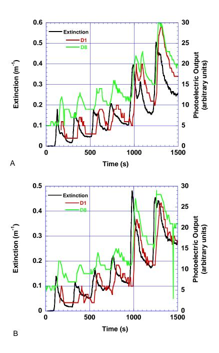
Figure 186. Photoelectric sensor response to cotton smolder smoke calibration test. A and B indicate repeated tests
