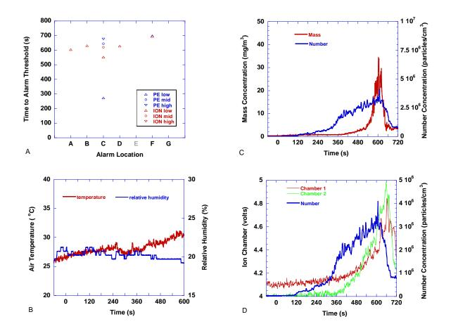
Figure 167. Broiling Pizza - one frozen pizza in oven set on broil, floor fan off. Oven on at t=0
