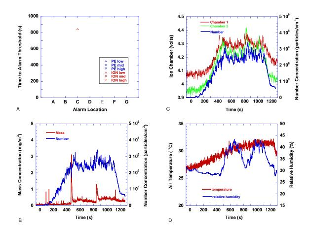
Figure 166. Deep-frying french fries scenario - steel wok, LPG hotplate, floor fan off, first french fries in pan at t=360 s
