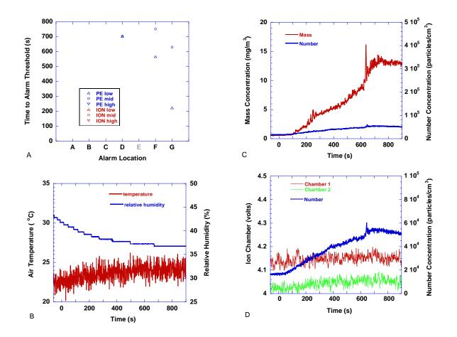
Figure 184. Smoldering foam - a polyurethane foam block, located on the living room floor at the chair burn location and ignited with an electrically powered nichrome wire heater imbedded in the block. Fan was on. Power to igniter on at t=0
