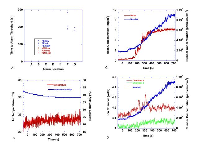
Figure 183. Smoldering foam - a polyurethane foam block, located on the living room floor at the chair burn location and ignited with an electrically powered nichrome wire heater imbedded in the block. Fan was off. Power to igniter on at t=0. Sample stopped smoldering
