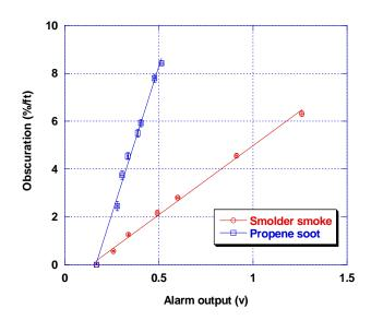
Figure 14. Calibration runs for Photo-1 alarm
