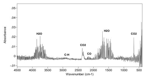
Figure 14. Average of spectra for fire room during the 50-s flaming in Test 4
