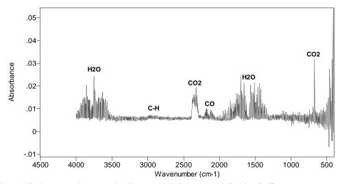
Figure 15. Average of spectra for fire room during the 60-s flaming in Test 6
