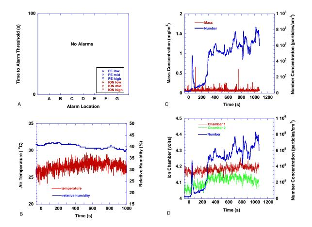
Figure 175. Candles burning - four tea candles burning on electric range top area. Floor fan was off. Candles lit at t=0
