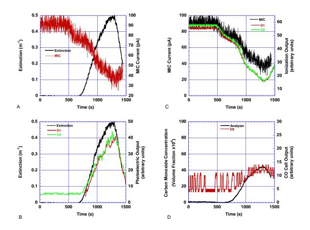
Figure 195. Smoldering wood fire scenario, fan speed 12 Hz
