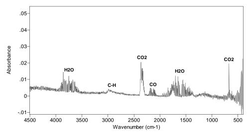
Figure 8. 4-min average of FTIR spectra (at 104 min) for master bedroom (Test 1)
