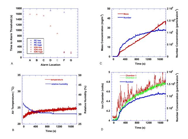
Figure 179. Smoldering cotton wicks -eight sets of four wicks were ignited with a 12 s delay using the staged wick ignition device, located on the living room floor at the chair burn location. Fan was on. Ignition sequence started at t=30 s
