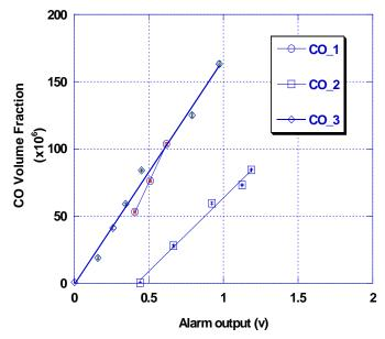
Figure 17. Calibration runs for CO alarms
