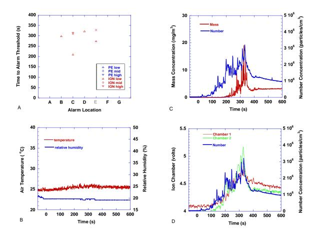
Figure 152. Toasting frozen bagel scenario - toaster on at t=0, off at 300 s. Room fan turned on
