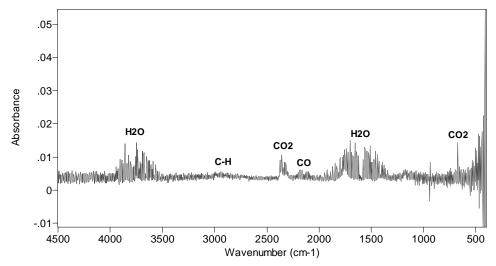
Figure 13. 1-min average of spectra for fire room after first smoke alarm in Test 8 with mattress smouldering
