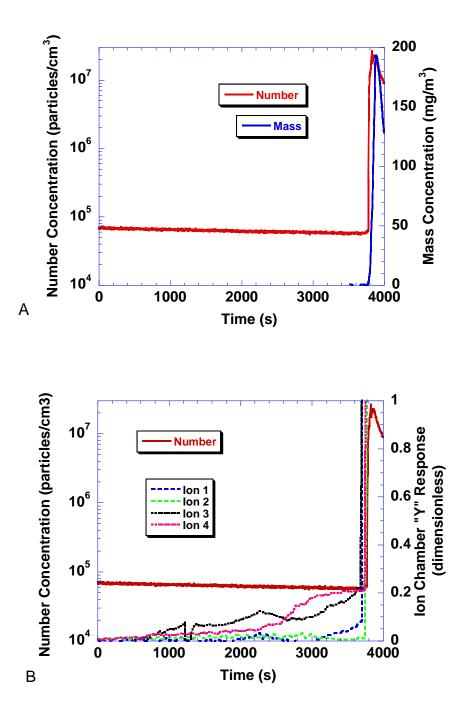
Figure 126. Smoke properties for smoldering mattress scenario SDC08
