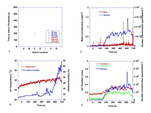
Figure173. Boiling spaghetti pasta - 2/3 package (300 g), floor fan off. Pasta placed in pot at t=450 s
