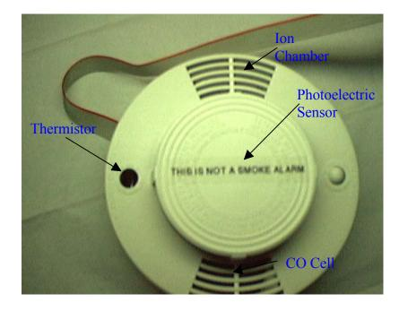
Figure 145. Photo, Ion, CO and thermistor unit
