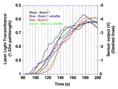
Figure 57. Ion-1 response, fan speed 7 Hz - repeat test
