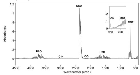
Figure 24. 30-s average of spectra for fire room after mattress flaming (Test 14)
