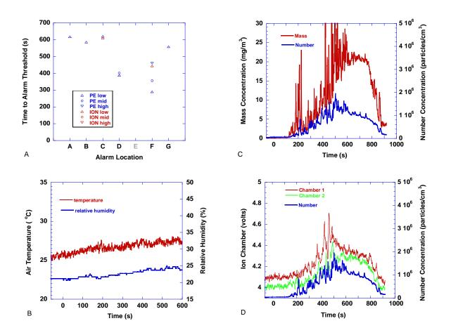
Figure 163. Frying hamburgers - three hamburgers in non-stick frying pan, floor fan on, living room window open. Hamburgers in pan at t=160 s
