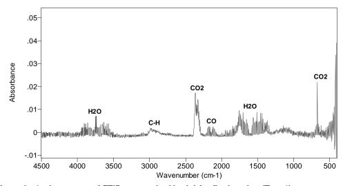
Figure 6. 4-min average of FTIR spectra (at 60 min) for fire location (Test 1)
