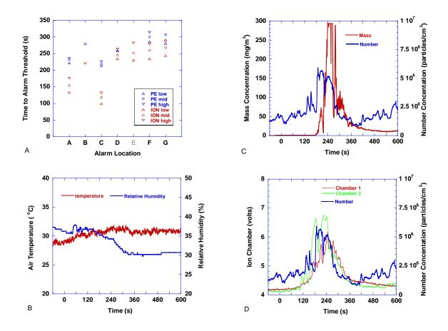
Figure 148. Toasting bread scenario – toaster on at t=0, off at 255 s. No forced flow, remote bedroom window open
