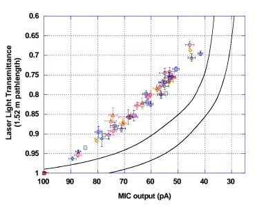
Figure 9. UL black smoke sensitivity limits and corresponding FE/DE data
