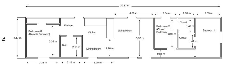
Figure 87. Layout of manufactured home used for test of smoke alarm performance
