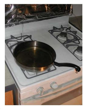
Figure 86. Heating ignition source with cooking oil
