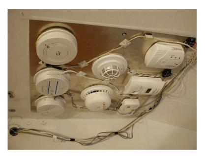
Figure 98. Measurement station showing several alarms arranged for testing
