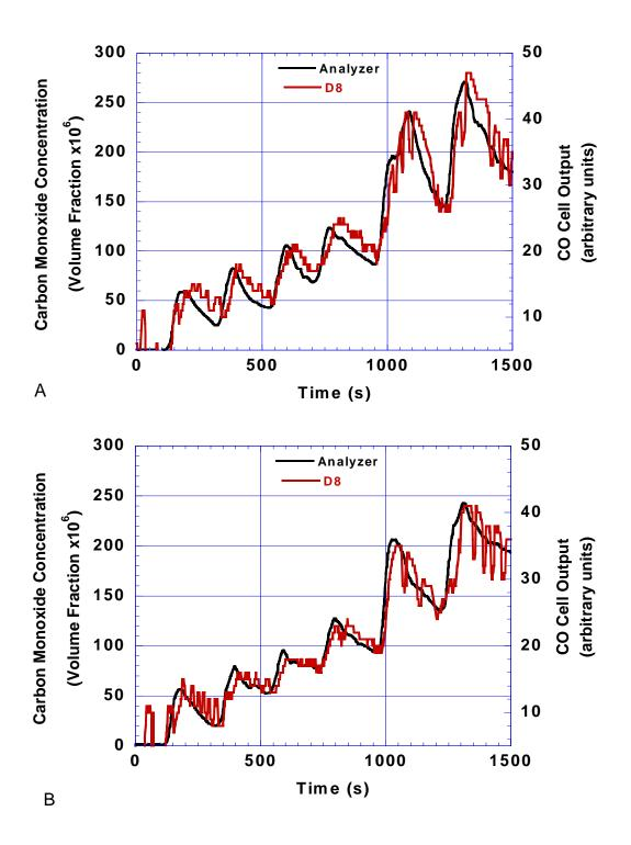
Figure 188. Electrochemical cell CO sensor response to cotton smolder smoke calibration test. A and B indicate repeated tests
