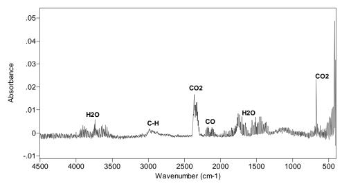
Figure 5. 4-min average of FTIR spectra for fire location after first smoke alarm (Test 1)
