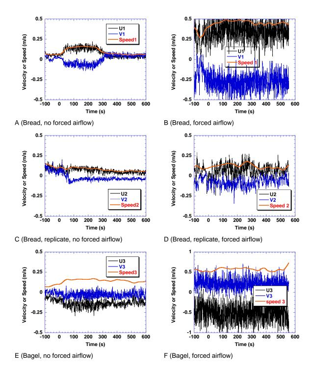
Figure 146. Velocity and speed components for toasting bread nuisance source with and without forced ventilation
