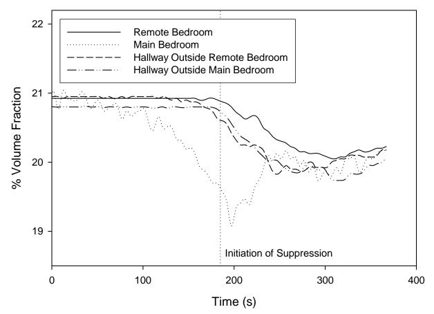
Figure 117. Oxygen concentration 900 mm below ceiling at four locations during a flaming ignition test of a mattress, test SDC05
