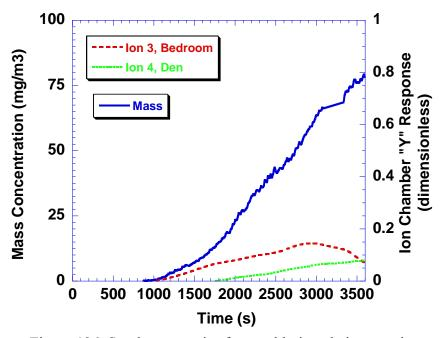
Figure 136. Smoke properties for smoldering chair scenario with air conditioning SDC27
