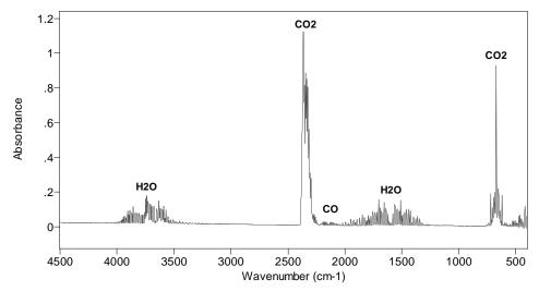
Figure 22. 2-min average of spectra for fire room after fire extinguishment (Test 9)
