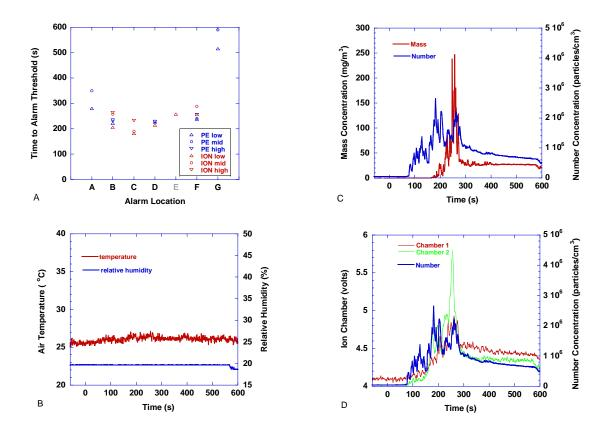
Figure 149. Toasting bread scenario - toaster on at t=0, off at 255 s. Room fan turned on
