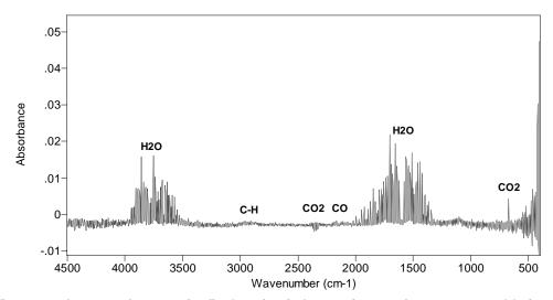
Figure 11. Average of spectra for fire location in last 4 minutes of mattress smouldering (Test 4)
