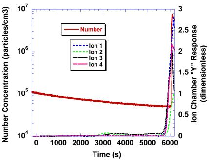
Figure 124. Smoke properties for smoldering mattress scenario SDC06
