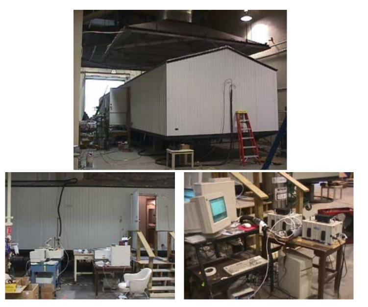
Figure 1. Manufactured home and FTIR measurement system
