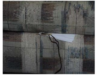
Figure 83. "Electric match" used for flaming ignitions
