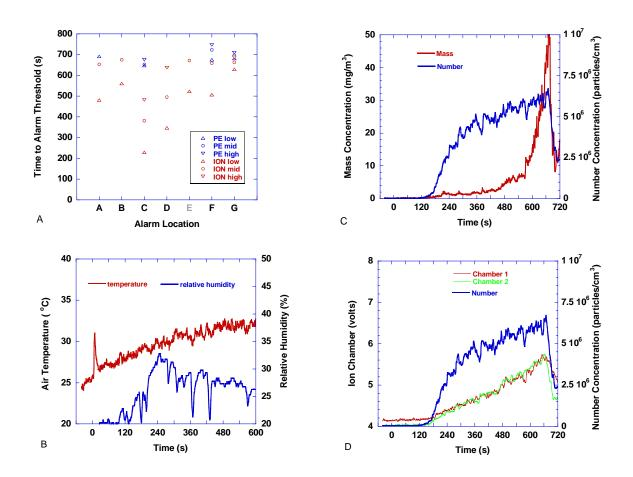
Figure 154. Frying bacon scenario - cast-iron pan, LPG hot plate, no forced flow, burner lit at t=0, bacon in pan at 60 s
