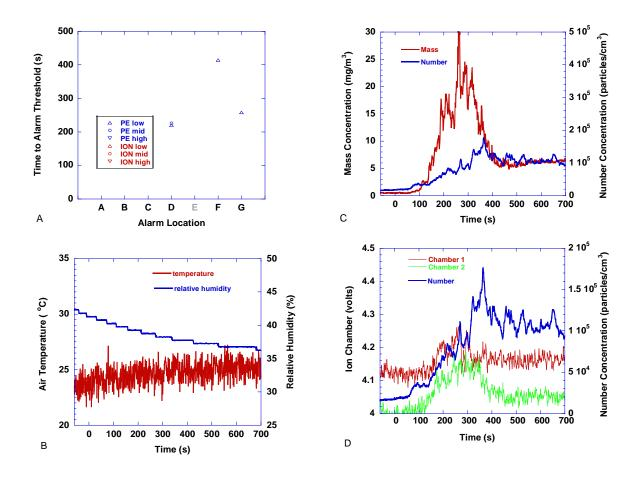
Figure 185. Smoldering foam - a polyurethane foam block, located on the living room floor at the chair burn location and ignited with an electrically powered nichrome wire heater imbedded in the block. Fan was on. Power to igniter on at t=0
