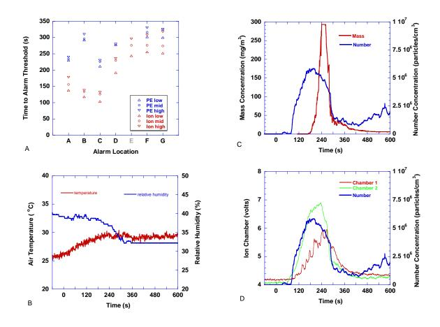
Figure 147. Toasting bread scenario - toaster on at t=0, off at 240 s. No forced flow
