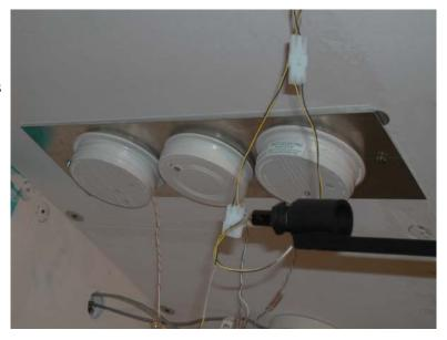
Figure 99. Measurement station showing unmodified smoke alarms arranged for testing
