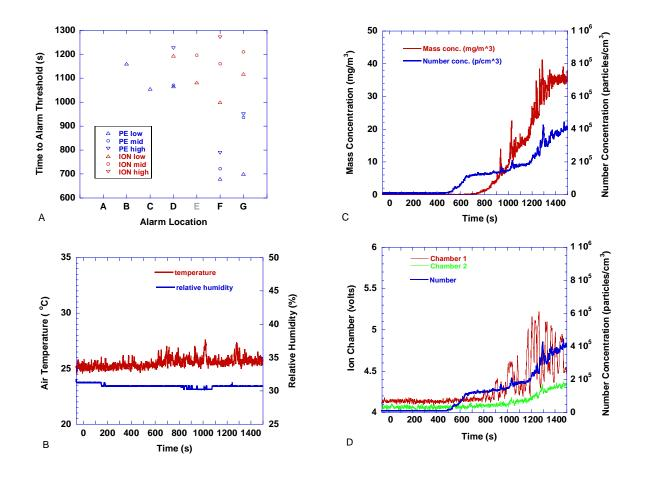
Figure 181. Smoldering wood blocks - eight beech wood blocks on an electric hotplate, located on the living room floor at the chair burn location. Fan was on. Power to hotplate on at t=0
