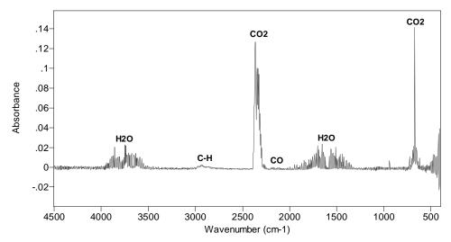
Figure 27. Average of spectra for last 2 minutes of cooking-oil heating (Test 13)
