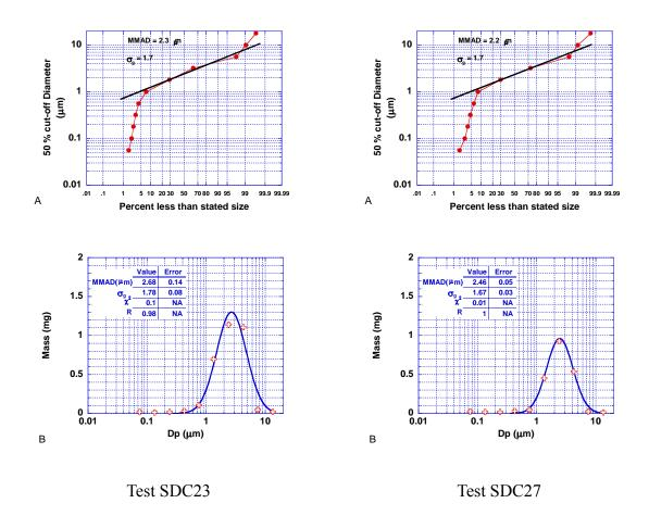
Figure 140. Cascade impactor results for smoldering chair fire scenarios SDC23 and SDC27
