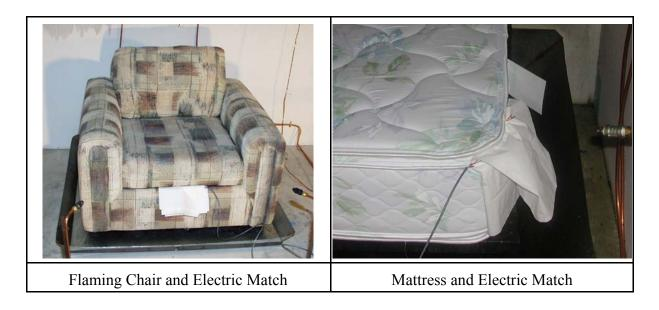
Figure 84. Location of "electric match" ignition source for flaming upholstered chair and mattress experiments
