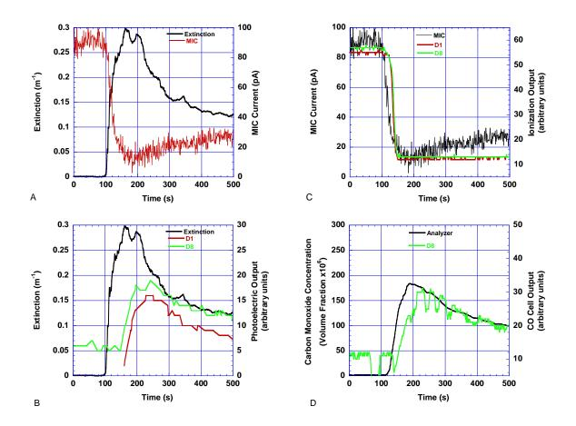
Figure 189. Smoldering cotton fire scenario, fan speed 7 Hz
