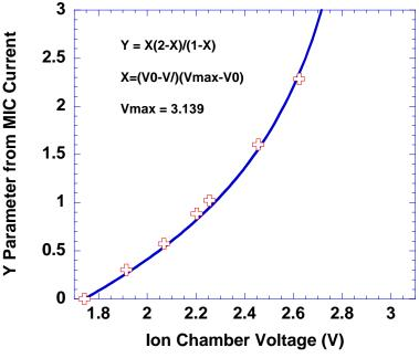
Figure 97. Calibration of residential ionization chamber
