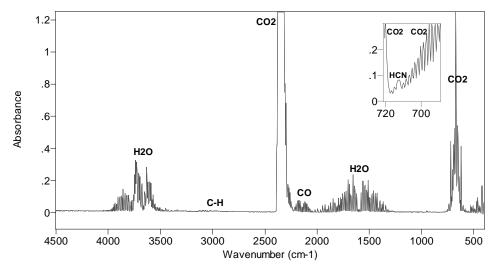
Figure 25. 90-s average of spectra for fire room after water spray (Test 14)
