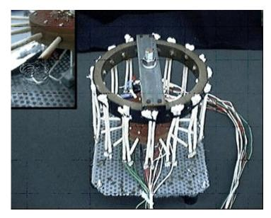
Figure 5. Smolder source, staged wick ignition device
