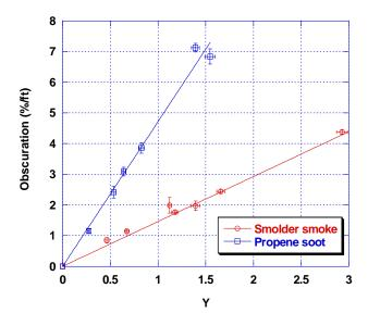
Figure 13. Calibration runs for Ion-4 alarm
