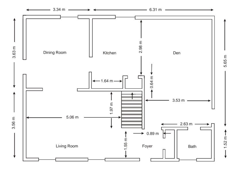
Figure 88. Layout of first floor of two-story home used for tests of smoke alarm performance
