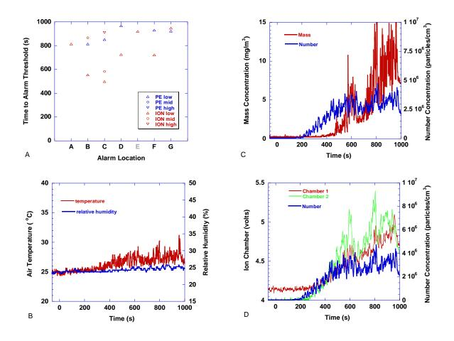
Figure 171. Broiling hamburgers - four hamburgers in oven set on broil, floor fan on. Oven on at t=0
