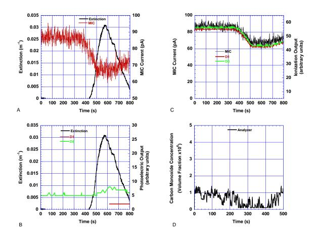
Figure 199. Margarine heated in a pan, fan speed 7 Hz
