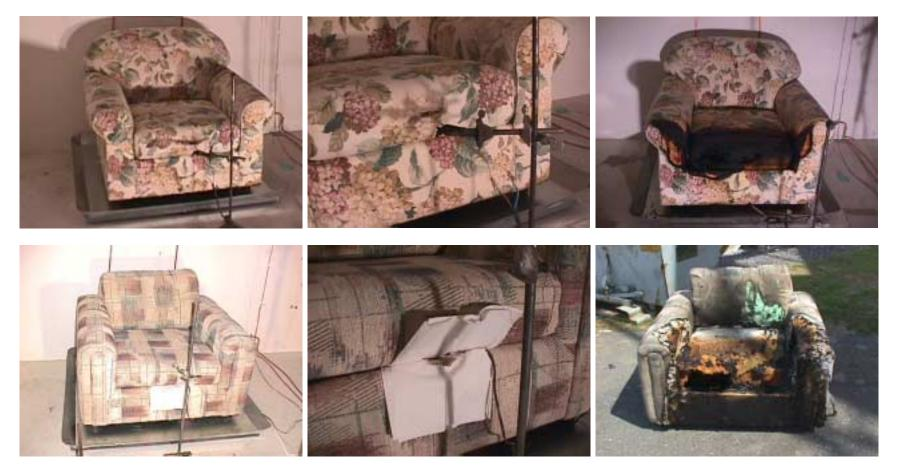
Figure 3. Upholstered chairs before and after smoldering (1<sup>st</sup> row) and flaming (2<sup>nd</sup> row) fire tests
