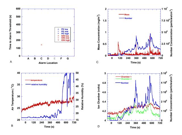
Figure 172. Boiling spaghetti pasta - 1/3 package (150 g), floor fan off. Pasta placed in pot at t=360 s
