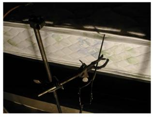
the polyurethane foam. Typical heat output was approximately 0.2 kW A thermocouple, Figure 85. Rod used for smoldering ignitions
