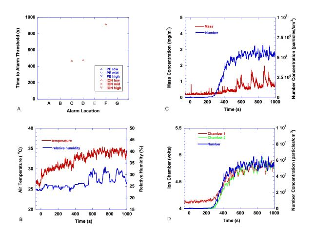
Figure 165. Deep-frying Tortillas scenario - steel wok, LPG hotplate, floor fan off, first tortillas in pan at t=360 s
