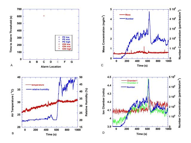
Figure 174. Boiling spaghetti pasta - 1/2 package (225 g), lid on, floor fan off. Pasta placed in pot at t=480 s
