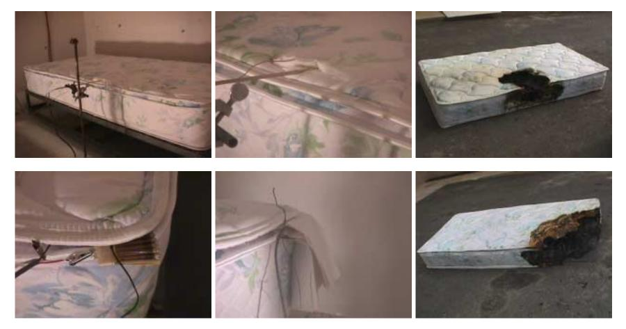
Figure 4. Twin-size mattresses before and after smoldering (1<sup>st</sup> row) and flaming (2<sup>nd</sup> row) fire tests
