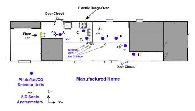
Figure 141. Schematic of the manufactured home for nuisance testing
